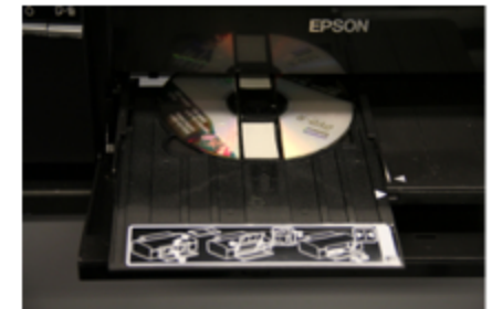
consumer inkjet printer with agar pad on CD tray
