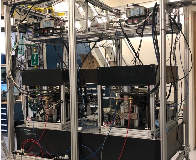
Two assembled Sr atom sources
