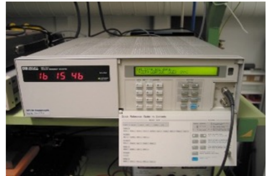
Cesium atomic clock since 1955 9.192.631.770 oscillations per second
